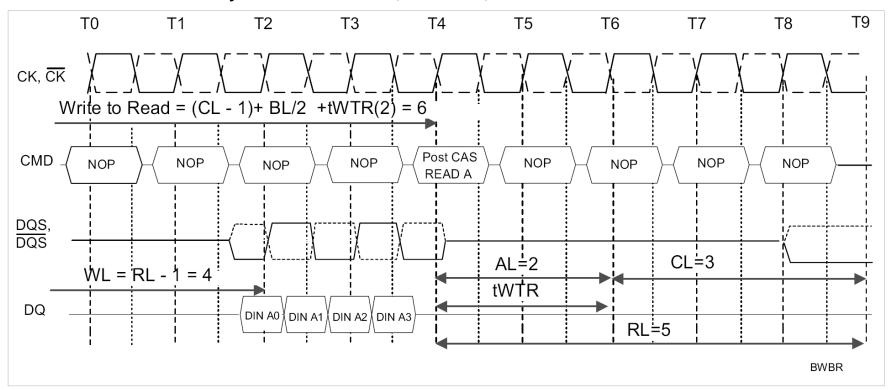
The minimum number of clocks from the burst write command to the burst read command is (CL - 1) +BL/2 + tWTR where tWTR is the write-to-read turn-around time tWTR expressed in clock cycles. The tWTR is not a write recovery time (tWR) but the time required to transfer 4 bit write data from the input buffer into sense amplifiers in the array.
