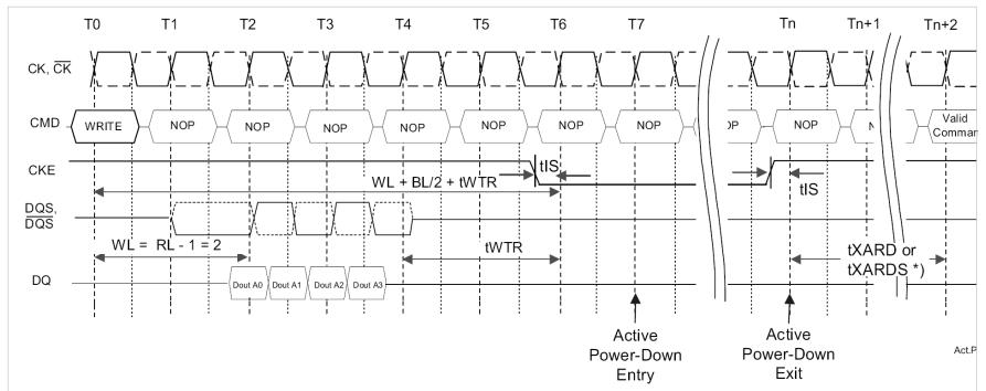
note: Active Power-Down mode exit timing tXARD ("fast exit") or tXARDS ("slow exit") depends on the programmed state in the MRS, address bit A12.
