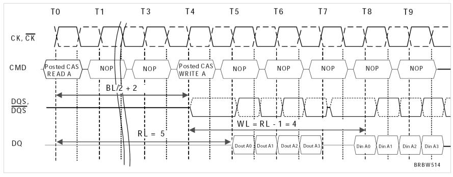
The minimum time from the burst read command to the burst write command is defined by a read-to-write turn-around time, which is BL/2 + 2 clocks.
