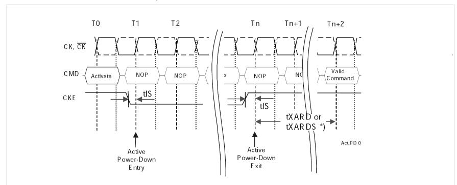
note: Active Power-Down mode exit timing tXARD ("fast exit") or tXARDS ("slow exit") depends on the programmed state in the MRS, address bit A12.
