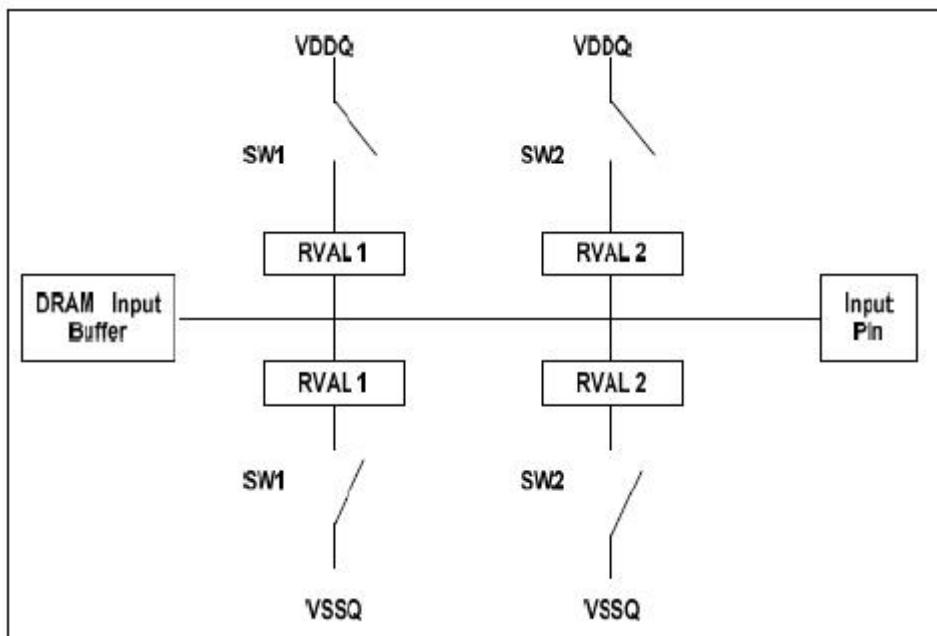
Switch sw1 or sw2 is enabled by the ODT pin. Selection between sw1 or sw2 is determined by "Rtt (nominal)" in EMRS(1) address bits A6 & A2. Target Rtt = 0.5 \* Rval1 or 0.5 \* Rval2.
