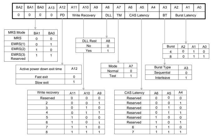
Note1. Active power down exit time's fast exit (A12=0) use t<sub>XARD</sub> and slow exit (A12=1) use t<sub>XARDS</sub>.
